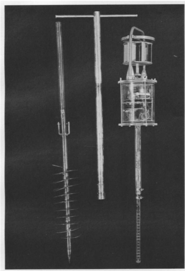
FIG. 3.—The "sedimeter" holder (with the transparent tube at the top), handle and instrument unit. The latter is equipped with an optional Savonius current rotor on top.
